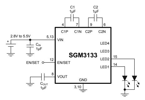
Figure 4. For 2-WLEDs Application Circuit
