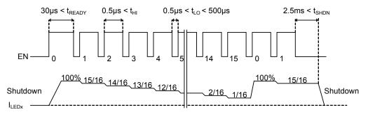
Figure 2. Brightness Control by Pulse Dimming
