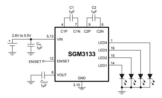
Figure 1. For 4-WLEDs Application Circuit
