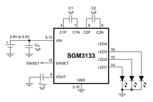
Figure 3. For 3-WLEDs Application Circuit
